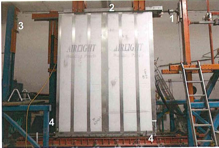
Figure 6 – Test Specimen Positioned in Test Frame (1) Load Cell, (2) Load Cap, (3) String Potentiometer, (4) Base LVDTs Two Panel – 96-in. long x 10-ft. tall x 5-1/2-in. thick assembly shown
