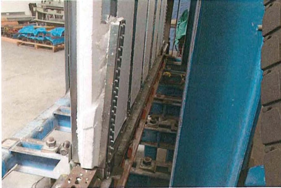
Figure 8 – Failure Mode (Observed in All Tests) Stud Fracture at the North-West Side of the Panel, Directly Above the Hold-Down
