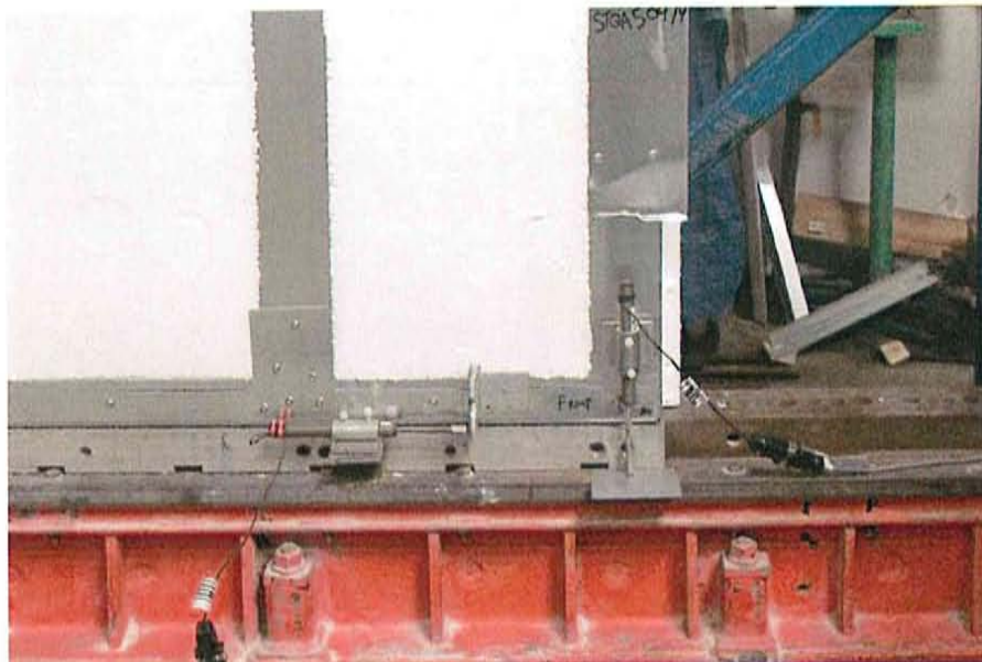
Figure 7 – Test Specimen Positioned in Test Frame – Close-up Horizontal and Vertical Deflection LVDTs
